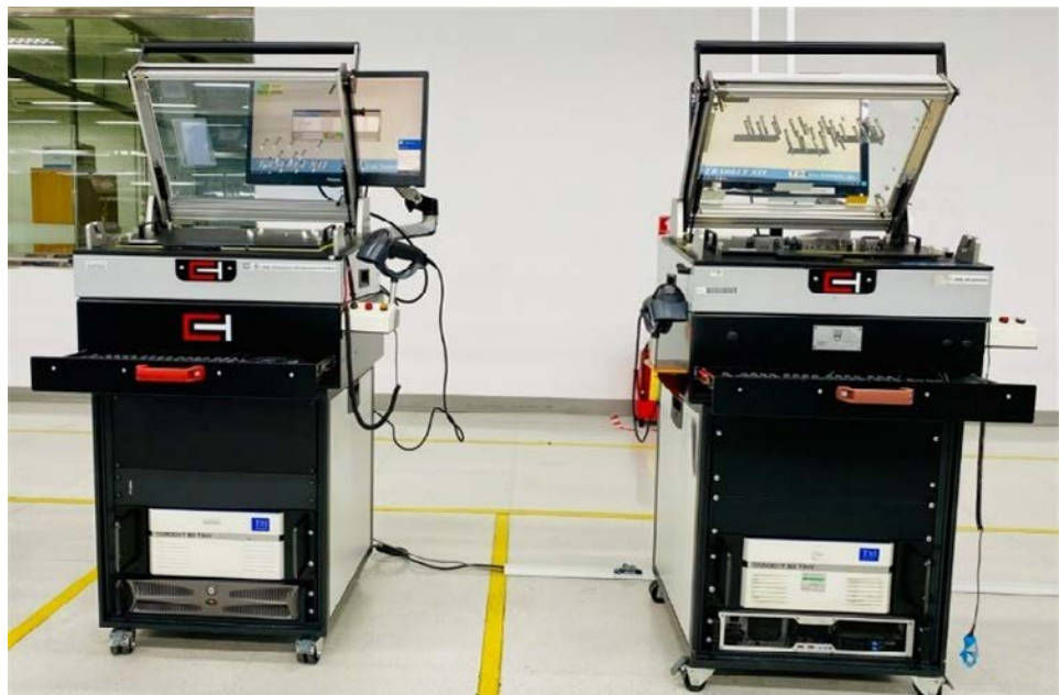
New TRI13 ICT Test system (left) adjacent to with TRI11 ICT Test system (right).
