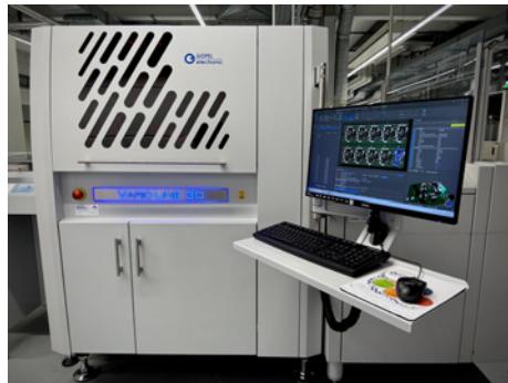
Neue AOI-Anlage Göpel Vario Line 3D X300
