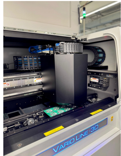
The heart of the AOI system: 3D/2D camera head
